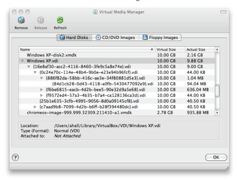
In all of these situations, from the point of view of the virtual machine, the virtual hard disk behaves like any other disk. While the virtual machine is running, there is a slight run-time I/O overhead because VirtualBox might need to look up sectors several times. This is not noticeable however since the tables with sector information are always kept in memory and can be looked up quickly.
