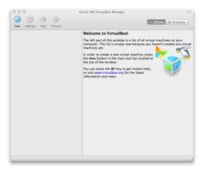
This window is called the "VirtualBox Manager". On the left, you can see a pane that will later list all your virtual machines. Since you have not created any, the list is empty. A row of buttons above it allows you to create new VMs and work on existing VMs, once you have some. The pane on the right displays the properties of the virtual machine currently selected, if any. Again, since you don't have any machines yet, the pane displays a welcome message.
