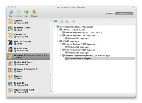
VirtualBox imposes no limits on the number of snapshots you can take. The only practical limitation is disk space on your host: each snapshot stores the state of the virtual machine and thus occupies some disk space. (See the next section for details on what exactly is stored in a snapshot.)
