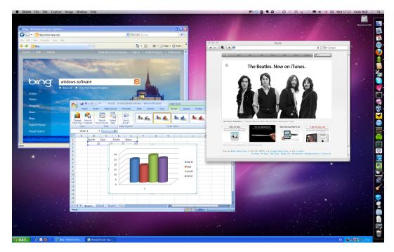
To enable seamless mode, after starting the virtual machine, press the Host key (normally the right control key) together with "L". This will enlarge the size of the VM's display to the size of your host screen and mask out the guest operating system's background. To go back to the "normal" VM display (i.e. to disable seamless windows), press the Host key and "L" again.
